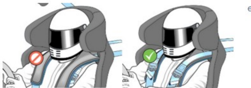
Fig. 16 - Example of incorrect and correct positioning of the harness straps when using a HANS®
