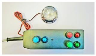
**The PZM-GPS safety tracking system installed in competing vehicle during the Rally** sends a signal to the Rally Control (RC). The system is activated automatically, so it doesn't need any operation before start and after finish the Special Stage.
